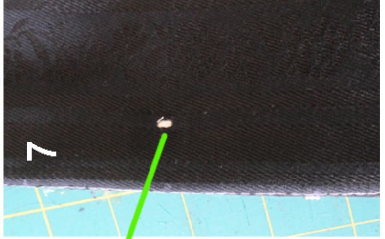
8 - Bar-tack on bars. Notice that there is an opening in the bar. The opening should go to the open end of the bodice back.
